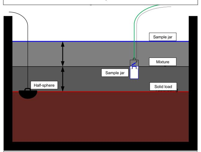
First you use the hemispherical sphere to determine the solid charge in the beun/hopper and the amount of water on top of the solid charge. Next, with the sample jar, you take a sample halfway into the mixture that is in suspension.
